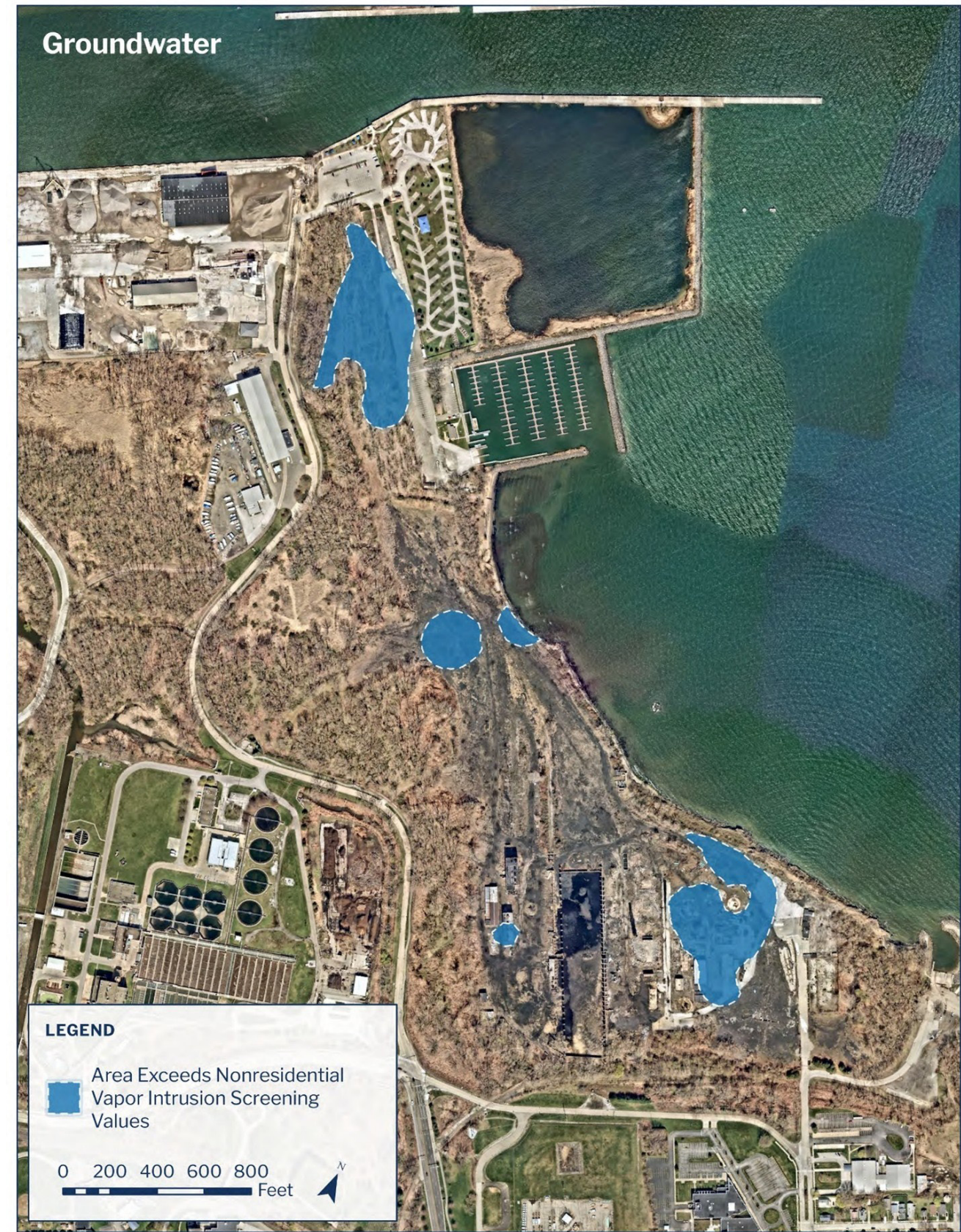
Figure 16: Vapor Intrusive Groundwater Contaminants
